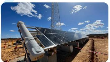
"It's a great system because it's a dry clean. An efficient clean using alternative wet methods can use 1-2 litres of water per panel and using water on hot panels during the day can cause cracking and damage to the panels."
